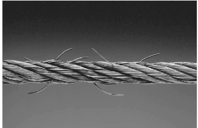
Cable With Broken Wires
